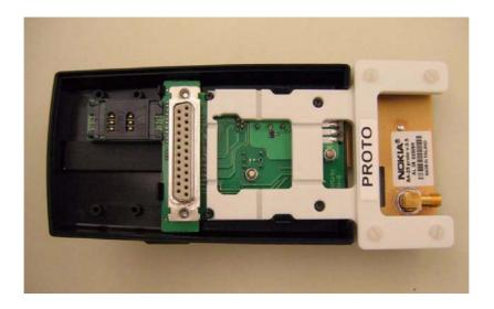
Close the docking station adapter by attaching the bottom plate.
