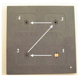
2. Once the best fit location has been found, leave the PA there and put the stencil on top of the jig and PA.
