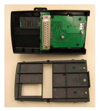
Remove the four screws fixing the PWB by using Torx T6 screw driver. These screws are too short, therefore four longer screws are delivered together with the coupler.
